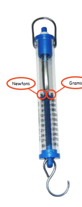
This is a FORCEMETER. Forcemeters are used to measure forces. Forces are measured in newtons. Some forcemeters also have readings in grams as they convert the force to a weight. Forcemeters have a hook at the bottom to attach to the object being measured and a spring inside. The spring stretches as the force is applied to the hook. The reading can then be taken where the spring stops to see what the force measurement is.
